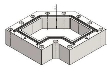
Each enclosure unit is designed to service a range of nominal pipe sizes (NPS) by simply machining the bore of the end caps to suit requirements.
